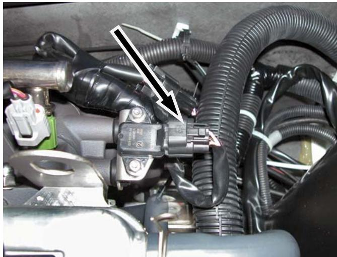
Install supplied Boost Clamp between stock map sensor and electrical connector.
