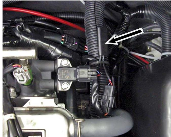
Secure map sensor to large hose using supplied zip tie.
